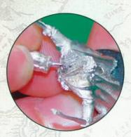
4 To make sure the holes line up, dab some paint on the end of the pin and line it up with the piece you want to drill. This will leave a small dot marking the area for you to drill.
