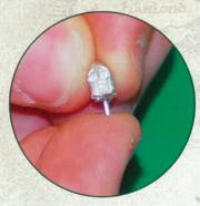
3 Superglue a short length of metal into one of the holes to act as the pin. A paper clip, or brass rod, is ideal for this.
