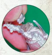
5 Drill the model as before. Then push the two parts together. The metal pin will strengthen the join, which leaves you to super glue the model together.
