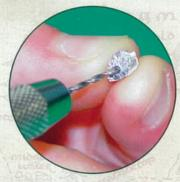
2 Next, use your pin vise to drill a hole into the model.
